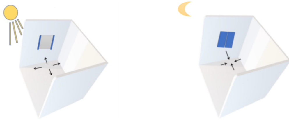
Figure 6: Thermal mass, absorbing and releasing heat
