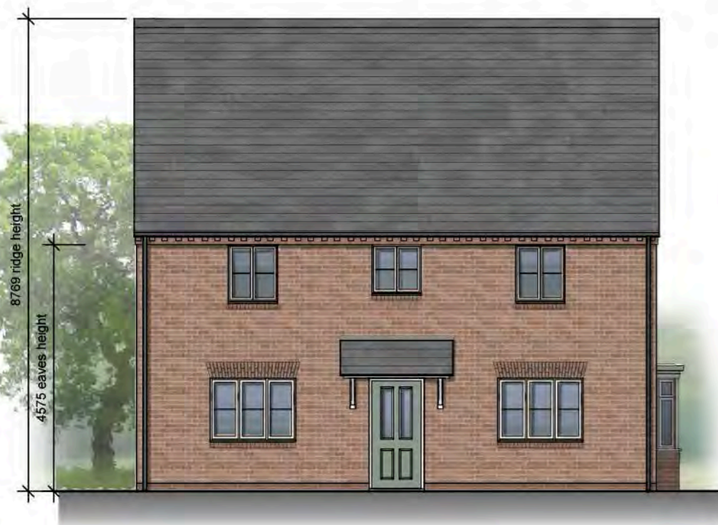
Side Elevation - Brick
