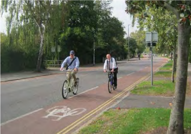
Figure 6.33: Red pigmented asphalt is used for all cycle routes in Cambridgeshire
