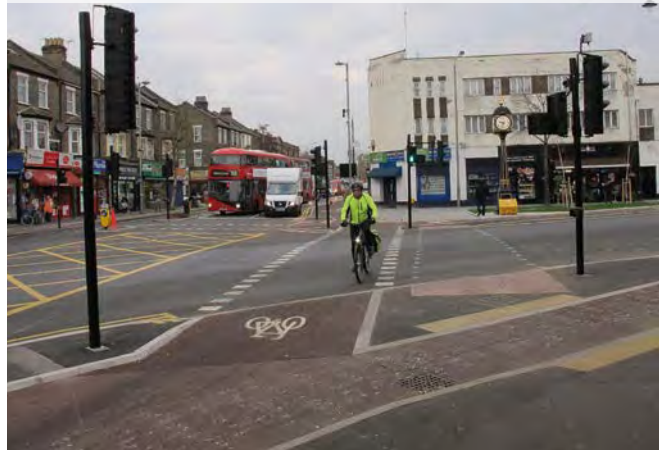
Figure 10.26: Circulating Cycle Stage Junction, Waltham Forest
