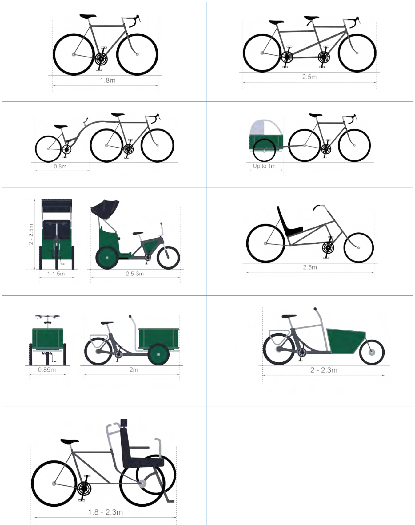
Figure 5.2: Typical dimensions of cycles
