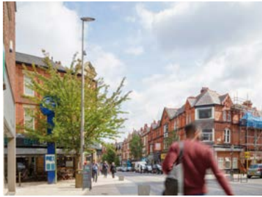
Streets 8-10m tall Lighting Column Distribution - approximately every 30m
