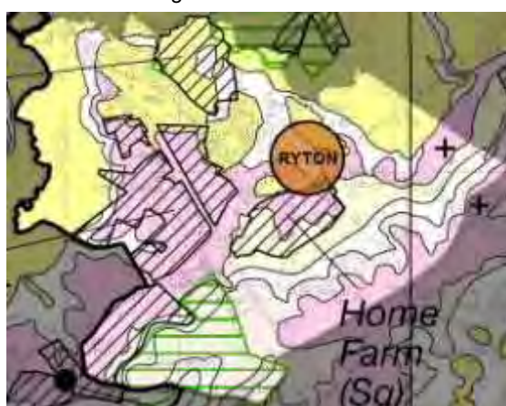
Figure 7: Ryton extract from Mineral Resources map (British Geological Survey, for Warks CC); Pink = sand and gravel. Hatched = worked out
